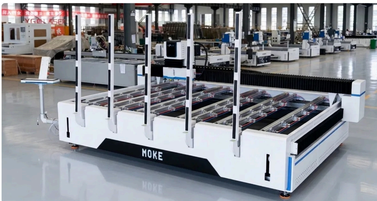
CF1530 with pneumatic loading arm and open-grid worktable
